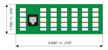
The above diagram shows the basic board layout for all boards in the economy series. In addition to the standard configurations, we can produce any board layout in this configuration with little or no tooling or set up cost based upon order quantities.
