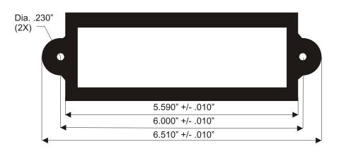
The above diagram shows the standard mounting frame dimensions for the economy series. It is designed to be used in a can with a 6.0" hole pattern using Richco SLPB-2M-B/SLG-2M-B Plungers/Grommets (included). See web site for specifications. Recommended mounting hole diameter .250"-.256". Can also be mounted using self drilling screws in cans without a matching hole pattern. Not what you need? Proto-Tel can design and mold custom brackets and produce custom PCBA's to meet any application.
